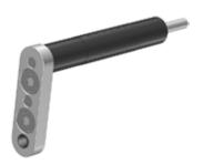
One of a kind drill attachment. Designed with a head thickness of only 7/16'' for drilling in areas as close as 1". Fits any air or electric drill. Accepts  $1/4 \times 28$  threaded drill bits and accessories for close quarter drilling. Dimensions are 6-5/8'' long, 7/16'' head thickness, 2-5/16'' offset distance, 7/16'' side to center. Drill capacity is 1/4''.
